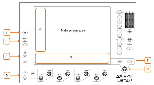
**Home** – Press to restore a familiar state of the Surface. Home restores default active layers, screen modes, active Mix, strip rotary mode and channel LCD view.
